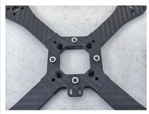
Start the stack assembly by installing the **Nylon Bolts** (D) through the inside holes in the corners. The bolts are held in place with a nylon nut as shown in the picture to the left.
