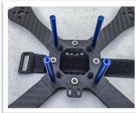
The battery strap can now be permanently installed. It is held in place using the **Battery Plate** (C) and **the M3 X 14mm Bolts** (J). The battery plate bolts will screw into the **40mm Standoffs** (C). This is another place where you can use thread-locking compound if desired.
