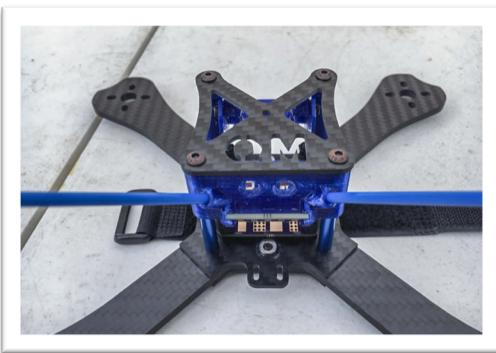
Once the receiver plate and the camera assembly have been installed you can install the **Top Plate** (D) using the **M3 X 8mm Bolts** (H). The cutout in the top plate faces the front of the frame.
