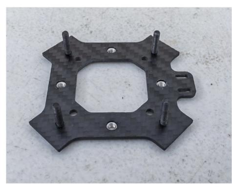
In order to facilitate the assembly of the frame we are temporarily going to use the **M3 X 14mm bolts** (J). Insert them into the **Main Plate** (A) in the outermost corner holes from the top-side (the side that has the nuts protruding) and place the plate top-side-down on a flat work surface. Once this is done your plate should look like the picture to the left.
