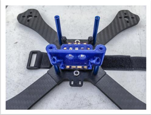
Slide the **Receiver, VTX, LED and Antenna Tray** (K) over the two rear standoffs (the ones closer to the power lead stress relief tab). This piece will hold all the listed components:
