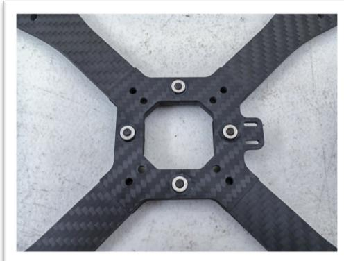
We can now remove the **M3 X 14mm bolts** (J) that were temporarily used to keep the sandwich together, they will be used later to mount the battery plate and the standoffs. The pictures above show what the main frame sandwich should look like from the bottom and from the top when completely assembled.
