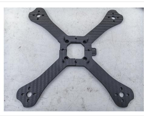
Place the **4mm Arms** (E) over the **M3 X 14mm bolts** (J), this will ensure that they are in the proper location. The arms should come together at the inside edges and the semi-circular notches will line up with the press-nuts that are in the main plate.
